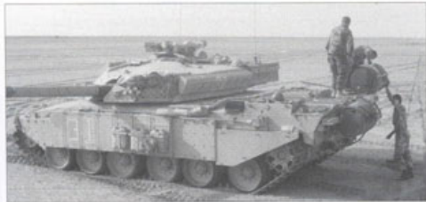
A further modification made to Challengers during Operation Granby was the fitting of two 45-gallon fuel drums at the rear. Here, the crew of a Challenger 1 Mark 3 of B Squadron Royal Scots Dragoon Guards manhandles a fuel drum into the 'upright position' for gravity feed of diesel into the main fuel tanks. This device increased the combat range by some 100 kilometres. (SCOTS DG)
