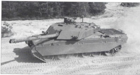
The final model of FV4030 developed for the Imperial Iranian Army was the Shir Iran 2, subsequently known as Shir 2, which was the first to feature the Hydrogas suspension system. One of the reasons for the demise of the FV4211 and the development of FV4030 was the insistence of the IIA on an all-steel tank, because of the problems of stress corrosion cracking associated with aluminium armour. (MOD)
