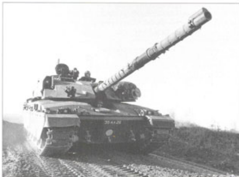
A Challenger 1 Mark 2 of 2nd Royal Tank Regiment moves off on a 'battle run' on the tank gunnery ranges at Hohné during 1989. With a high reputation for gunnery, 2 RTR failed the cut for CAT '87 which was to have far reaching ramifications to the future of Challenger. Here, the L11AS 120mm with its thermal shield is shown to advantage. (MOD)
