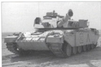
With the armoured door of the TOGS barbettes open, a Challenger 1 Mark 3 of The Queen's Royal Irish Hussars displays the full array of supplementary armour fitted to the Challengers of 1st (UK) Armoured Division during Operation Granby, with Chobham armour panels along the sides and Explosive Reactive Armour (ERA) on the glacis plate and toe. (QRH)
